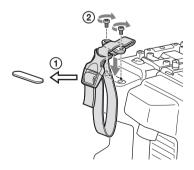
**3** ① Release the buckle, ② bundle the cable with the belt, ③ then lock the buckle again.
