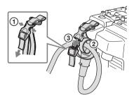
4 Adjust the length by pulling down the end of the belt.
