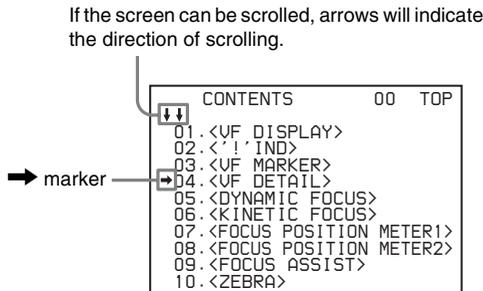
Turn the MENU SEL knob/ENTER button to align the arrow marker (➡) to the page to be set and press the MENU SEL knob/ENTER button.
