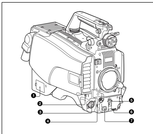
**1 NETWORK TRUNK connector (RJ-45 8-pin)**
