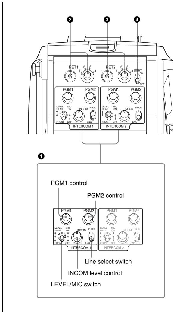
**1 INTERCOM1 and INTERCOM2 controls and switches**
