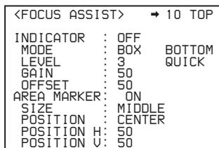
**3** Turn the MENU SEL knob/ENTER button to align the arrow marker (➡) to the item to be set and press the MENU SEL knob/ENTER button.
